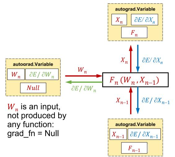
$F_n$ contains boththe data forward function $X_n = F(W_n, X_{n-1})$ and the gradient backwardfunction(s) $\frac{\partial E}{\partial X_{n-1}} = \frac{\partial E}{\partial X_n} \cdot \frac{\partial F(W, X_{n-1})}{\partial X_{n-1}}$  $\frac{\partial E}{\partial W_n} = \frac{\partial E}{\partial X_n} \cdot \frac{\partial F(W_n, X_{n-1})}{\partial W_n}$
