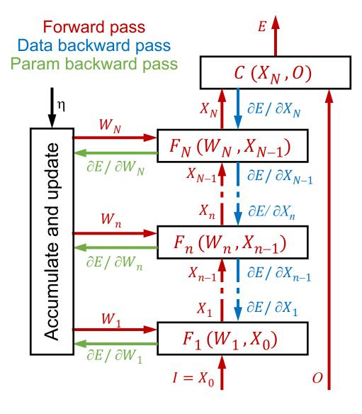
Forward pass, for  $1 \le n \le N$ :  $X_n = F_n(W_n, X_{n-1})$  $E = C(X_N, O)$
