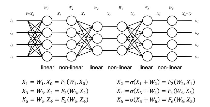
$O = (F_6(W_6) \circ F_5(W_5) \circ F_4(W_4) \circ F_3(W_3) \circ F_2(W_2) \circ F_1(W_1))(I) = (o_{n=1}^{n=6} F_n(W_n))(I)$
