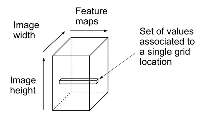
Input image data is a special case with 3 feature maps corresponding to the RGB planes and sometimes 4 or even more for RGB-D or for hyper-spectral (satellite) image data.
