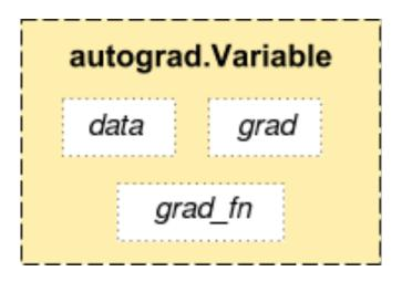
Define  $X_n = F_n(W_n, X_{n-1})$  for  $1 \le n \le N$  (or arbitrary network) End with  $E = C(X_N, O)$ Execute a forward pass for a training sample (I, O)Call E.backward() (backward pass from *E* with  $\partial E / \partial E = 1$ ) Get all  $\partial E / \partial W_n$  (and  $\partial E / \partial X_n$ ) for that training sample
