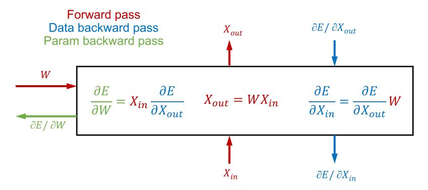
Note:  $X_{in}$  and  $X_{out}$  are regular (column) vectors and W is a matrix while  $\partial E / \partial X_{in}$ and  $\partial E / \partial X_{out}$  are transpose (row) vectors (this is because  $dE = (\partial E / \partial X) . dX$ ).  $\partial E / \partial W$  is a transposed matrix which is the *outer* product of the regular and transpose vectors  $X_{in}$  and  $\partial E / \partial X_{out}$ .
